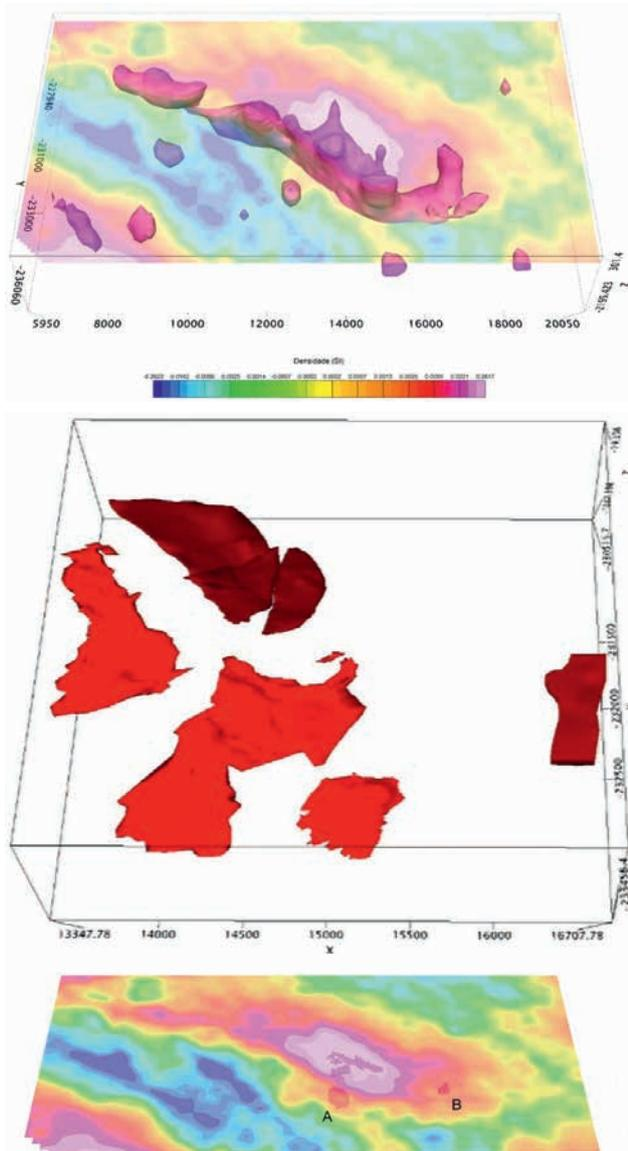
**Figure 4** Top: Density model produced in the unconstrained inversion (density differences in  $\text{g/cm}^3$ ), overlaid to the Bouguer anomaly map. Middle: 3D model of the massive sulphide lenses based on drill-hole data used to constrain the 3D gravimetric inversion. Bottom: Density model produced using the 3D geological model above as a constraint (density differences in  $\text{g/cm}^3$ ) overlaid on the Bouguer anomaly map.
