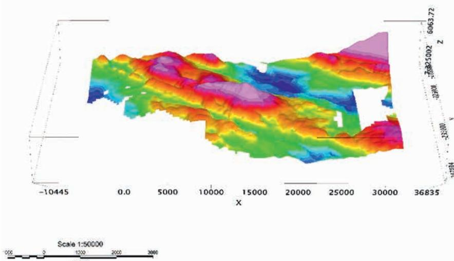
**Figure 3** 3D view of the residual Bouguer anomaly map used for the study area, extracted and relevelled from the IPB Portuguese sector gravity map shown in Figure 2. Reference density of 2.6 g/cm<sup>3</sup> for the Bouguer anomaly calculation and a second degree polynomial was used to produce the residual (Marques et al., 2019).
